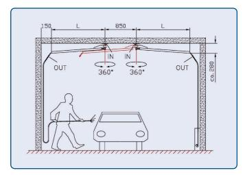
**Application example:** The arrangement of two gyroscopes allows very comfortable washing of vehicles. 1 gyroscope for high pressure, 1 additional gyroscope for the foam brush, ensures entire rational mobility. Minimum distance is 850mm.
